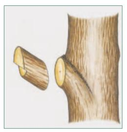
**Fig. 53:** If there is no discernible branch collar, a cut must be made outside the branch bark ridge, but parallel to the trunk, rather than at a slant, as with a stub cut. This prevents both the formation of a nourishment blind spot at the lower wound margin and dieoff in the area generally.
