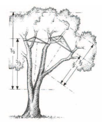
**Fig. 66.:** The height of installation for a single-level fracture prevention system (ZTV-Baumpflege 2006).
