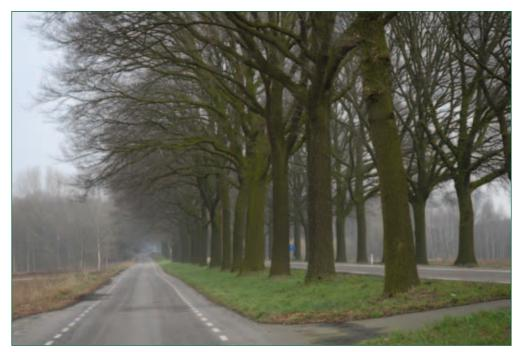
Fig. 33: To accomplish clearance for traffic of 4.2 m, it will in many cases be necessary to achieve a clear trunk height of 6 metres.
