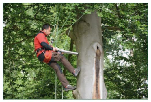
**Fig. 40:** This beech tree with a large pruning wound and symptoms of internal decay in the temporary crown is analysed with a resistograph. Pruning at the right time could have prevented these problems. The total costs of one tree risk assessment like this, including a report, amount in general up to twice the overall costs of pruning a young tree during a period of 25 years!
