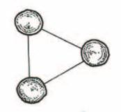
**Fig. 67:** Direct connection between two limbs/stems. Lateral swaying of secured crown parts is not obstructed (ZTV-Baumpflege 2006).
