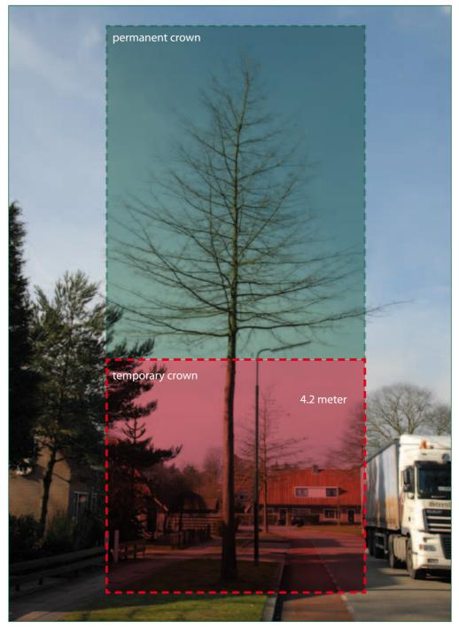
**Fig. 32:** In this situation clearance for traffic should be minimum 4.2 m. The actual height of branch-free trunk is 5.0 m. This is to assure that the clearance of 4.2 m will be maintained also in the future with branches leaning down.
