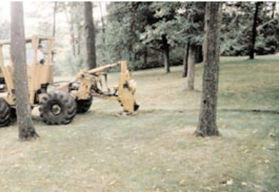
One method of controlling the spread of Oak Wilt is through root graft disruption. This involves cutting roots with a trencher or rock saw
